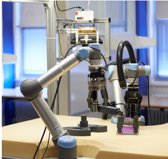
Fig. 1. Marvin platform assembling the Cranfield benchmark.
